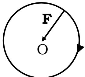
$$\alpha = \frac{d\omega}{dt} = 0 \quad (\omega = \text{일정})$$
